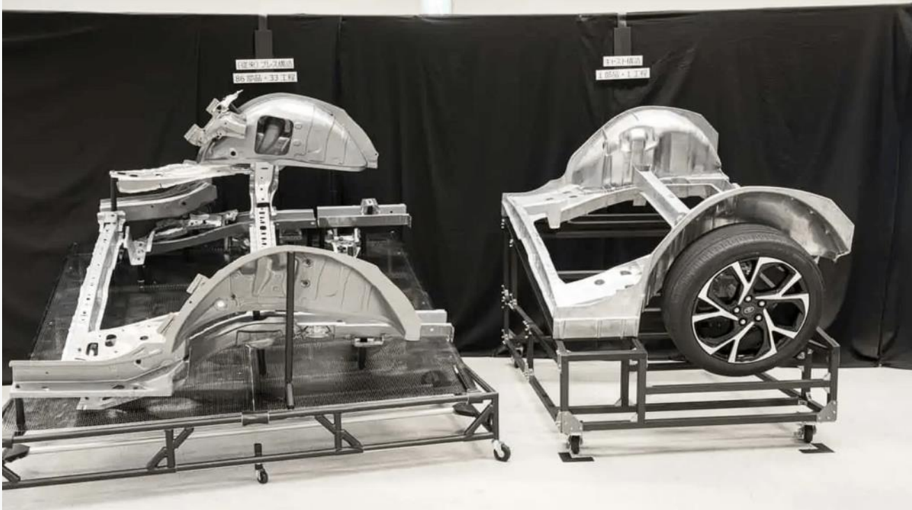
Toyota Gigacasting Old (Left) vs New (Right)
